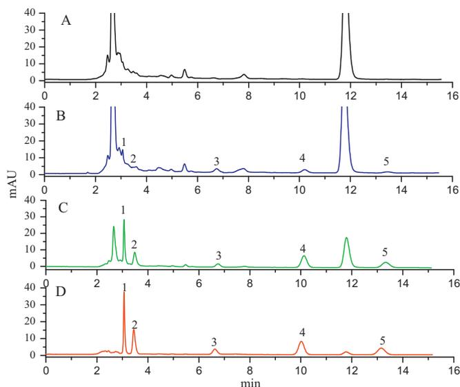
**Fig. 12.** Chromatograms of five water-soluble acid dyes in different water samples. Raw wastewater sample (A), spiked wastewater sample (B), spiked wastewater sample after a clean-up on SAX-SPE (C), and spiked wastewater sample after a clean-up on 1-MA-3MI-Br-mag-MIPs (D). Peak 1: tratarzine; Peak 2: amaranth; Peak 3: Orange G; Peak 4: Brilliant ponceau 5R; Peak 5: Sunset Yellow FCF.
