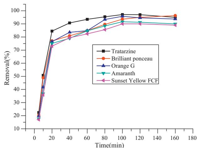
**Fig. 9.** Removal kinetic curves of 1-MA-3-MI-Br-mag-MIPs toward water-soluble acid dyes. Conditions: 1.0 g sorbent, 50 mL of 100 mg/L mixture of water-soluble acid dyes, shaking time 3 h, temperature 25 °C.
