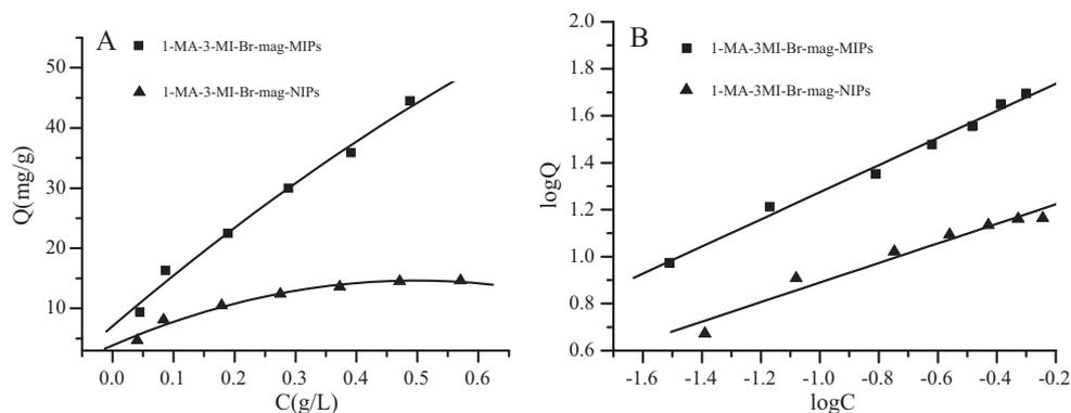
Fig. 6. Adsorption isotherm of tritarzine on 1-MA-3MI-Br-mag-MIPs and 1-MA-3MI-Br-mag-NIPs (A) and fitting to the Freundlich isotherm (B). Conditions: 0.1 g sorbent, 50 mL of tritarzine, shaking time 2 h, temperature 25 °C.
