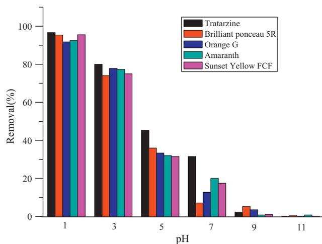
**Fig. 7.** Removal efficiency of 1-MA-3-MI-Br-mag-MIPs toward water-soluble acid dyes in different pH conditions. Conditions: 1.0 g sorbent, 50 mL of 100 mg/L mixture of water-soluble acid dyes, shaking time 2 h, temperature 25 °C.
