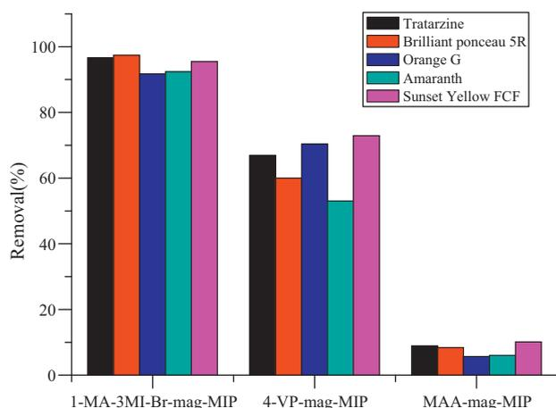
**Fig. 10.** Removal efficiency of three different sorbents toward water-soluble acid dye. Conditions: 1.0 g sorbent, 50 mL of 100 mg/L mixture of water-soluble acid dyes, shaking time 2 h, temperature 25 °C.
