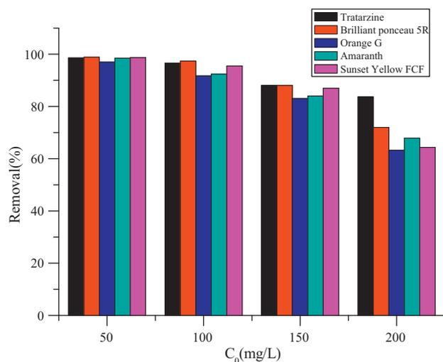
**Fig. 8.** Removal efficiency of 1-MA-3-MI-Br-mag-MIPs toward water-soluble acid dyes in different concentrations. Conditions: 1.0 g sorbent, 50 mL mixture of water-soluble acid dyes, shaking time 2 h, temperature 25 °C.
