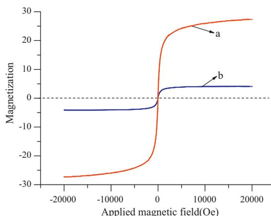
Fig. 4. VSM magnetization curves of PEG– $\text{Fe}_3\text{O}_4$  and 1-MA-3-MI-Br-mag-MIPs (a: PEG– $\text{Fe}_3\text{O}_4$ ,  $S_s$  saturation magnetization is 31.43 emu/g; b: 1-MA-3-MI-Br-mag-MIPs,  $S_s$  saturation magnetization is 4.06 emu/g).
