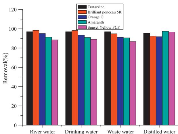
**Fig. 13.** Removal efficiency of 1-MA-3MI-Br-mag-MIPs toward different kinds of water. Conditions: 1.0 g sorbent, 50 mL of 100 mg/L mixture of water-soluble acid dyes, shaking time 2 h, temperature 25 °C.
